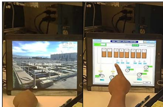
HMI flat panel touch-screens fitted with System 800xA graphics and animations.
