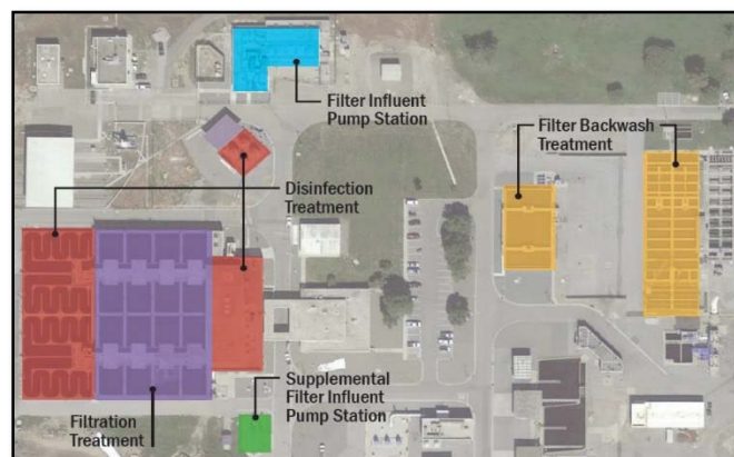
Filtration process is comprised of five process elements.
