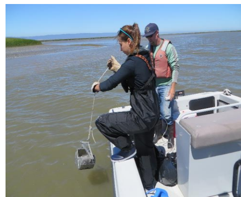
Jessica Donald collecting a benthic sample using a Ponar grab device.
