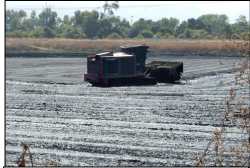
A lone FECON mulcher churning biosolids in a drying bed on 17 July, 2017.
