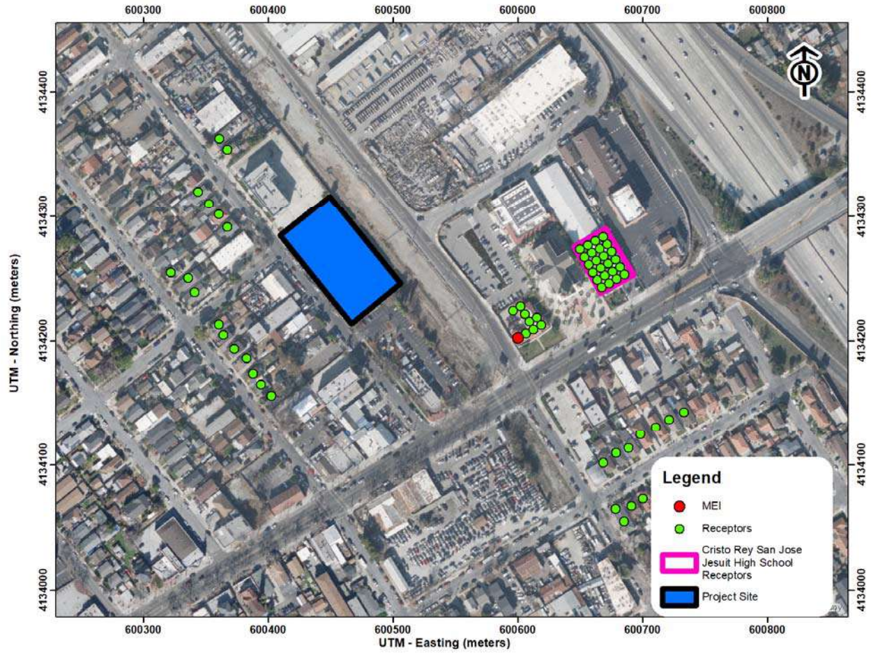
Figure 1. Locations of Project Construction Site, Off-Site Sensitive Receptors, and Maximum TAC Location (MEI)
