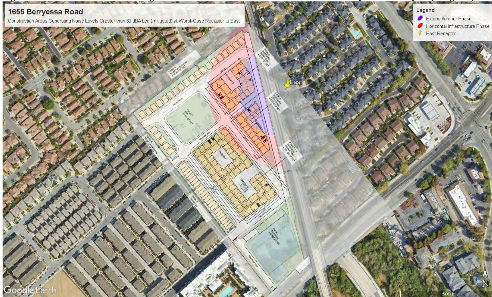
Figure 3 Areas of Site Generating Construction Noise Levels Greater than 60 dBA Leq at East Receptor (mitigated)
