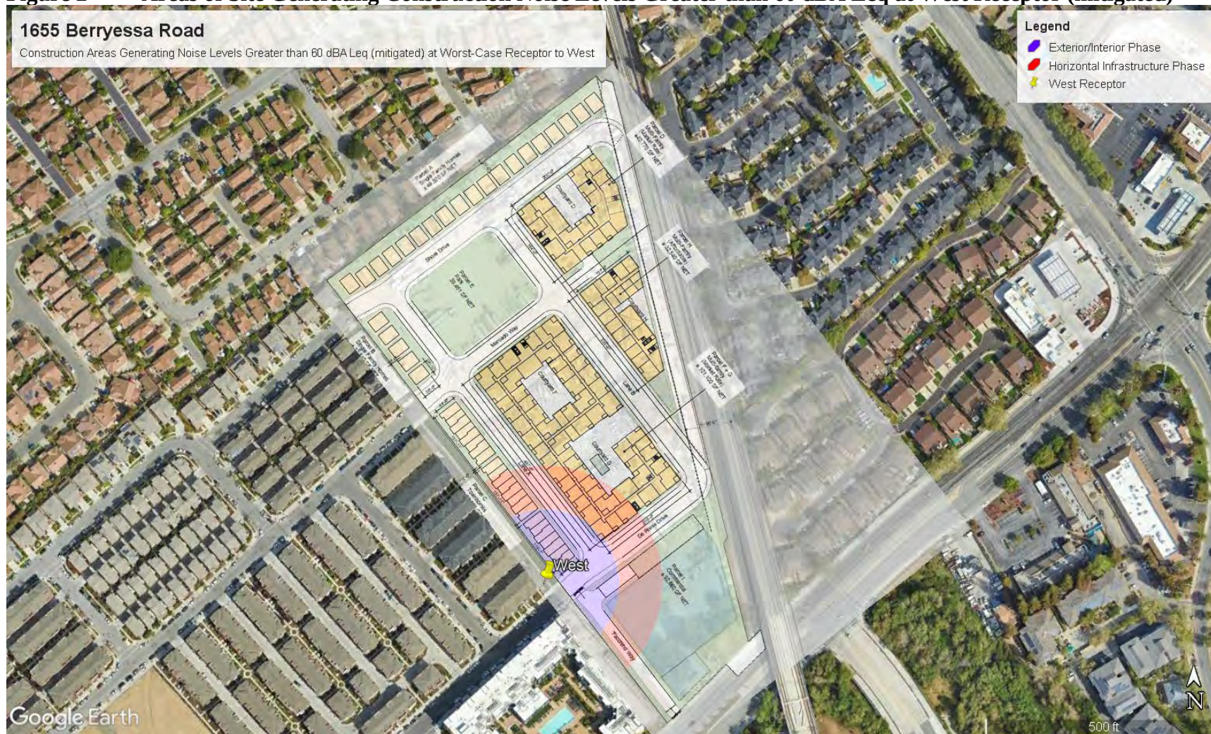
Figure 2 Areas of Site Generating Construction Noise Levels Greater than 60 dBA Leq at West Receptor (mitigated)
